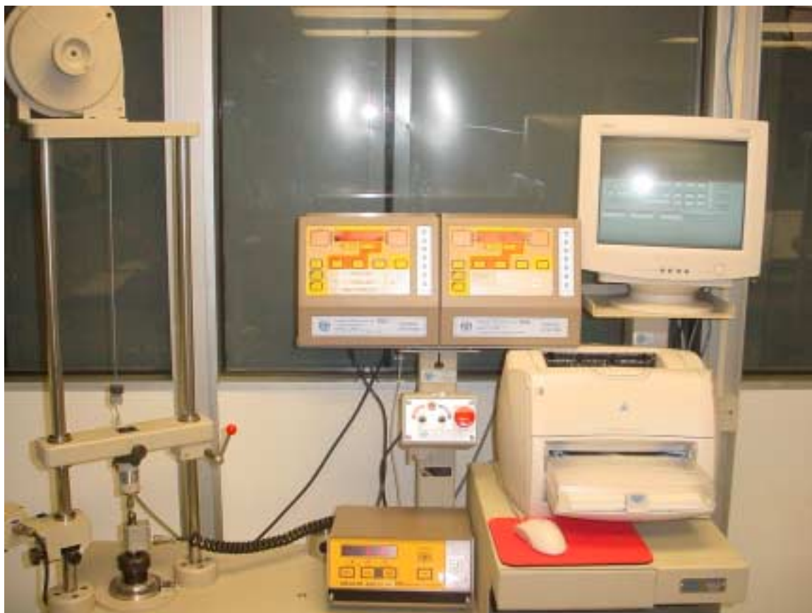
Figure 2. Automatic Test Equipment to Test for Locking Torque, Breakaway Torque, Preload & Torque-Off
